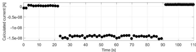
Fig. 12. Calculated current using Eq. 1 for output voltage results presented in Fig. 4.
