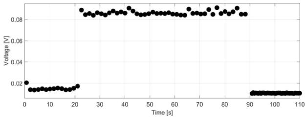
Fig. 6. Output voltage profile at irradiation dose rate of 3.1 mGy/s for 30 V reverse polarization.
