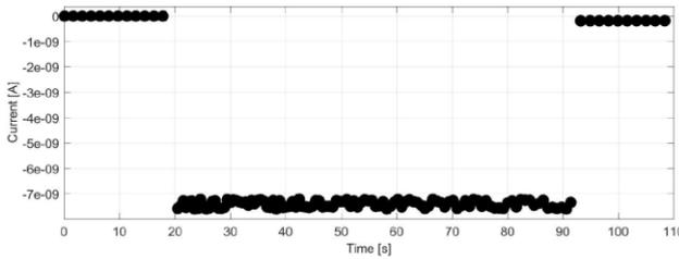
Fig. 7. Induced photocurrent profile at irradiation dose rate of 3.1 mGy/s for 30 V reverse polarization.
