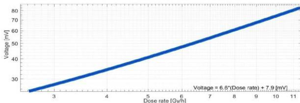
Fig. 13. Output voltage versus dose rate
