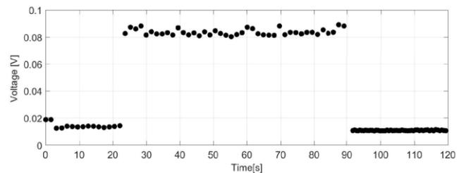
Fig. 4. Output voltage profile at irradiation dose rate of 3.1 mGy/s for 15 V reverse polarization.
