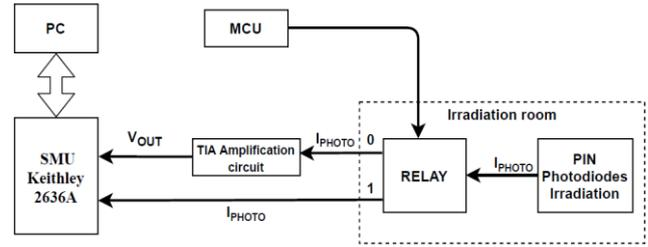
Fig. 3. Experiment setup block diagram.
