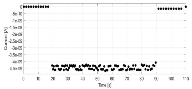
Fig. 9. Induced photocurrent profile at irradiation dose rate of 2.1 mGy/s for 15 V reverse polarization.
