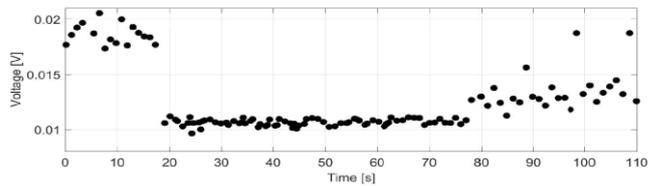
Fig. 10. Output voltage profile at irradiation dose rate of 0.28 mGy/s for 15 V reverse polarization.
