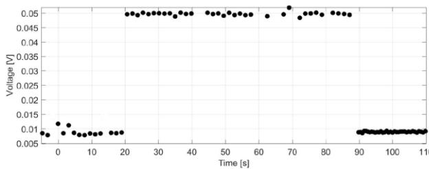
Fig. 8. Output voltage profile at irradiation dose rate of 2.1 mGy/s for 15 V reverse polarization.
