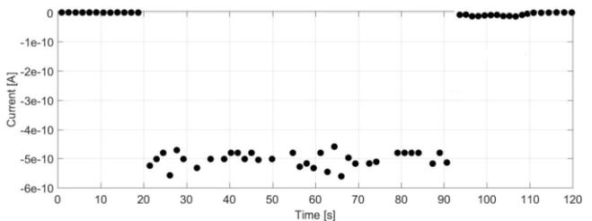
Fig. 11. Induced photocurrent profile at irradiation dose rate of 0.28 mGy/s for 15 V reverse polarization.
