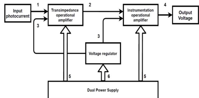
Fig. 1. Transimpedance amplifier circuit block diagram design.
