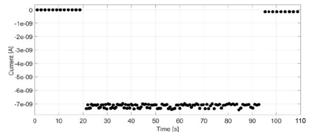
Fig. 5. Induced photocurrent profile at irradiation dose rate of 3.1 mGy/s for 15 V reverse polarization.
